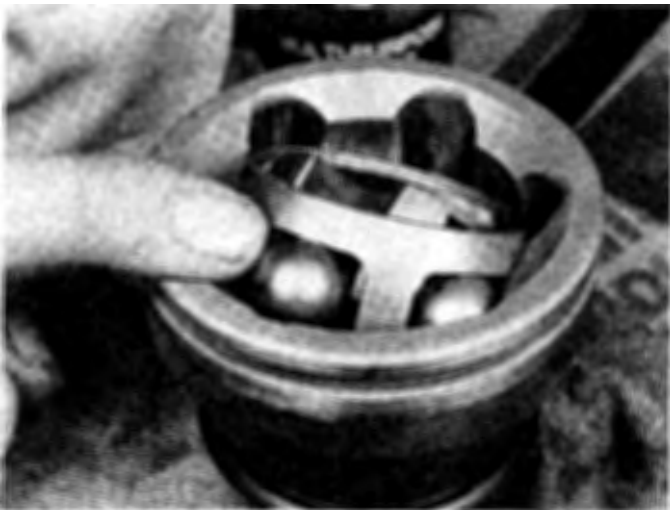
16.18 Align the cage windows and the inner and outer race grooves, then tilt the cage and inner race to insert the balls
