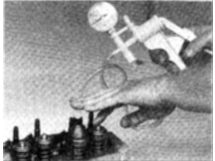
11.8 A special adapter and vacuum pump are required to check the O-ring valve stem seals for leaks
