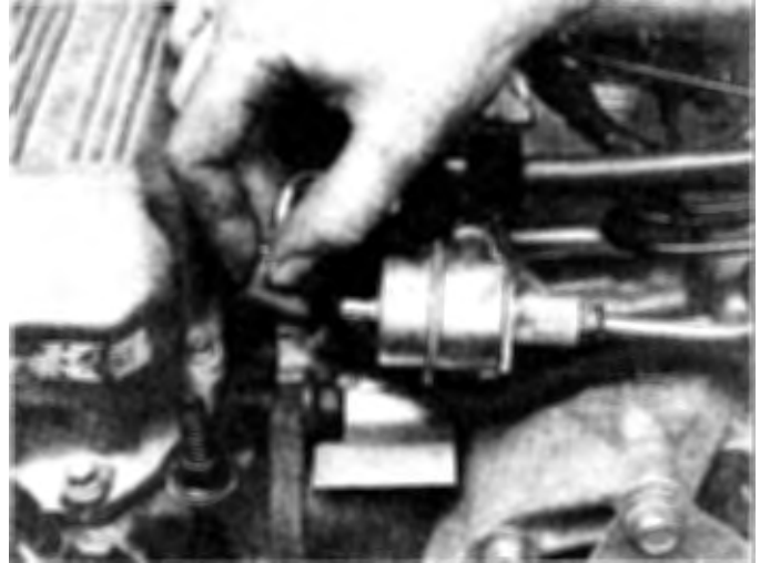
3.36 Detach the vacuum tube from the fuel pressure regulator, start the vehicle and note the gauge reading — with the vacuum line detached, fuel pressure should be about 39 psi
