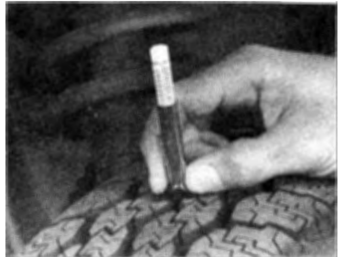
5.2 A tire tread depth indicator should be used to monitor tire wear — they are available at auto parts stores and service stations and cost very little
