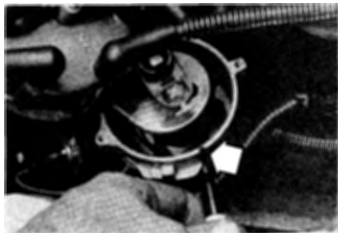
3.1c . . . then remove the distributor cap and verify that the rotor is pointing at the mark (arrow)
