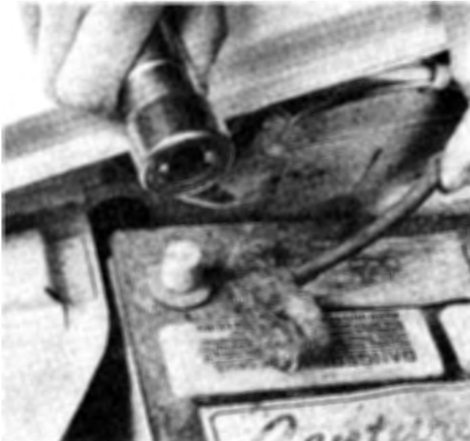
8.8c Regardless of the type of tool used to clean the battery posts, a clean, shiny surface should be the result
