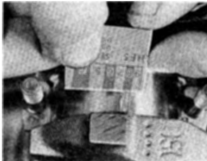
24.17 Measuring the width of the crushed Plastigage to determine the rod bearing oil clearance (be sure to use the correct scale — standard and metric scales are included)
