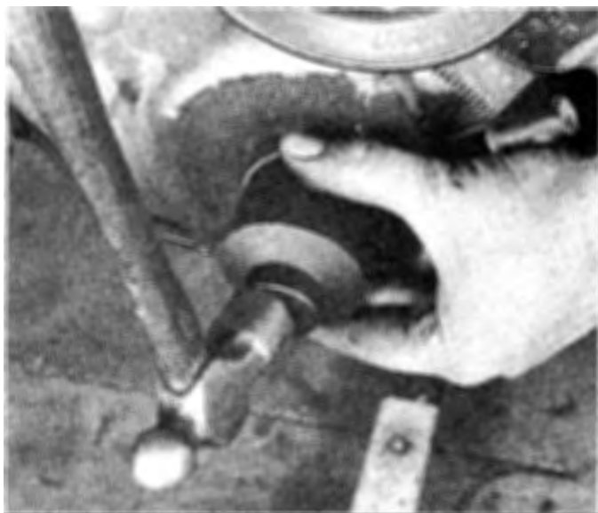
11.3 Gently drive the new seal into place with a hammer and large socket
