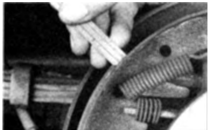
20.12 The lining thickness of the rear brake shoe is measured from the outer surface of the lining to the metal shoe
