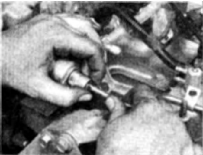
15.23c . . . then detach the fuel return line from the fuel pressure regulator
