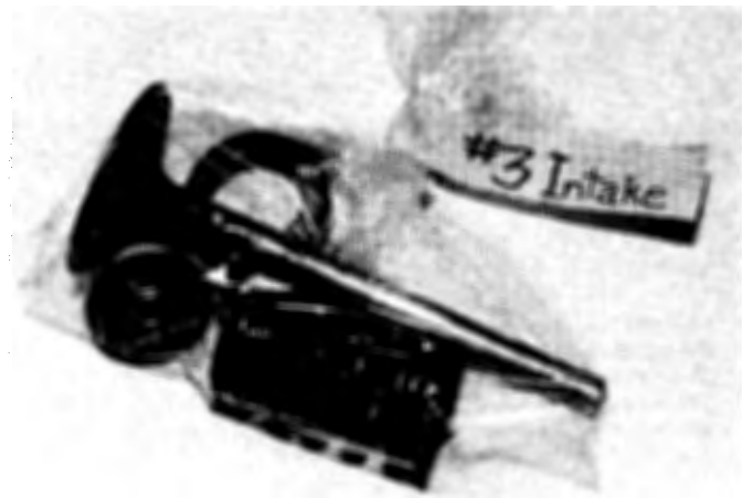
8.2 A small plastic bag, with an appropriate label, can be used to store the valve train components so they can be kept together and reinstalled in the correct guide
