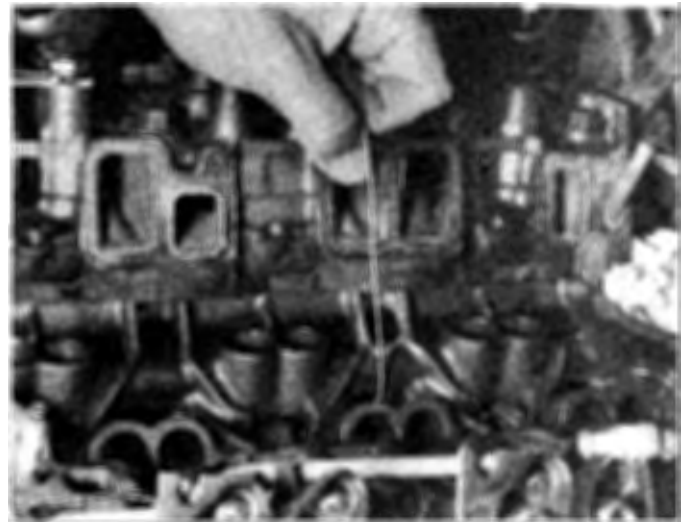
16.11 A length of wire with a hook on it can be used to support the camshaft as you guide it out of the block
