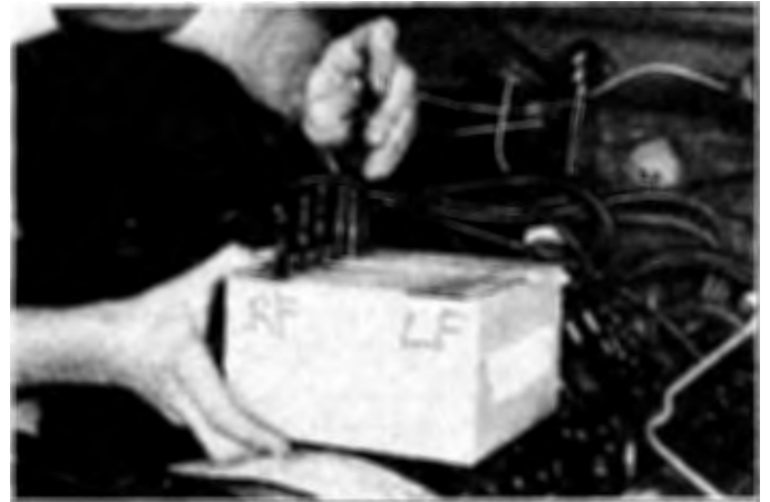
5.4 When removing the pushrods, be sure to store them separately to ensure reinstallation in their original positions
