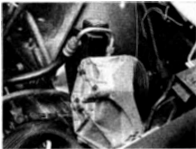
5.11 Set the power steering pump aside with the lines still connected — be sure it's upright so fluid won't spill
