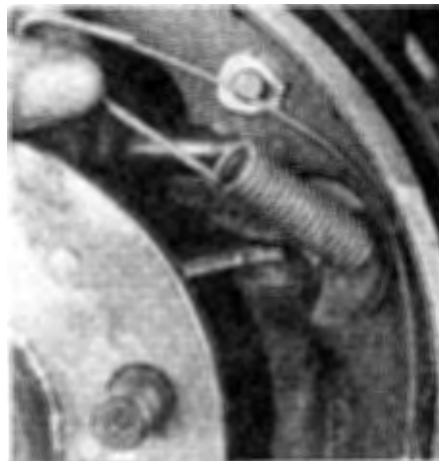
6.4t Hook the end of the secondary shoe retractor spring through the cable guide and into the hole in the shoe, then stretch the spring over the anchor pin
