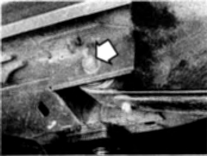
11.7 Remove the spring front eye-to-frame bracket bolt (arrow)
