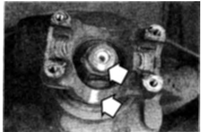
14.6a Mark the relationship of the pinion shaft to the pinion shaft yoke
