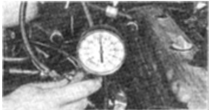
3.6 A compression gauge with a threaded fitting for the spark plug hole is preferred over the type that requires hand pressure to maintain the seal
