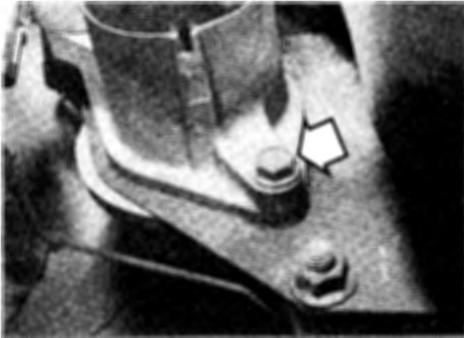
21.4a Lower starter mounting bolt (inline six-cylinder model shown) - view is from the rear, looking forward
