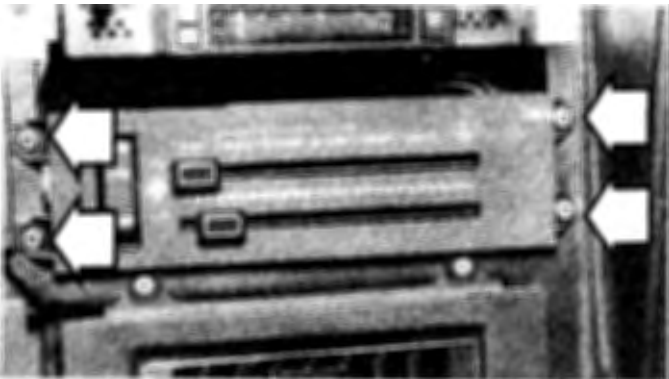
16.4 Remove the four air conditioning control panel mounting screws (arrows)
