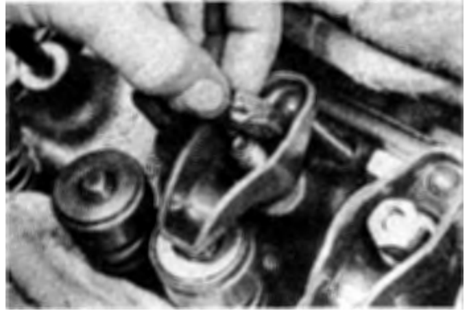
5.11 Moly-base grease applied to the pivot balls will ensure adequate lubrication until oil pressure builds up when the engine is started
