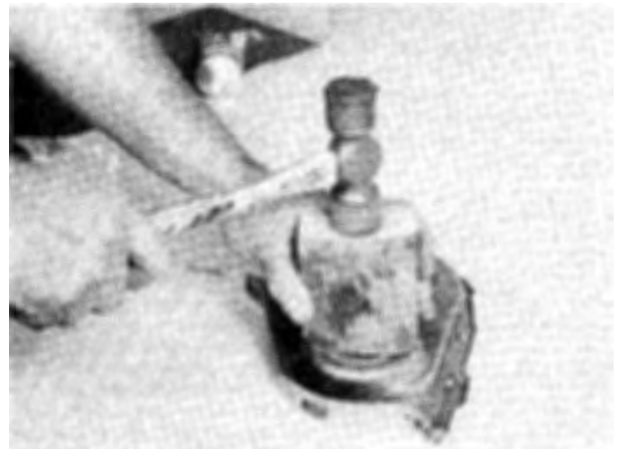
12.8b . . . or a block of wood and a hammer – don't damage the seal in the process!
