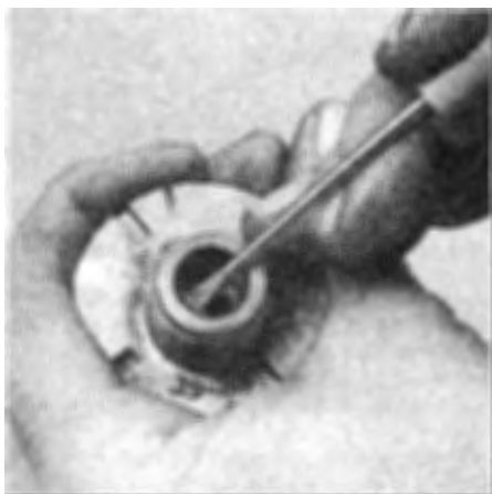
2.13b . . . then lift the adapter seal from the inside of the housing
