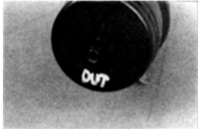
31.16 Make sure the word OUT on the fuel filter faces the engine
