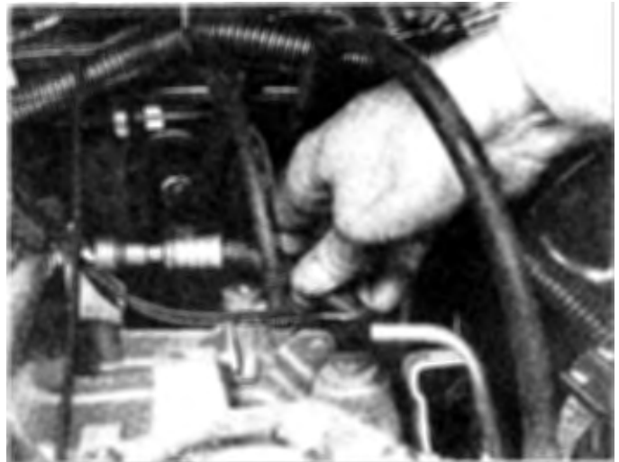
3.41 If the fuel pressure is below the specified level, momentarily pinch off the hose section of the fuel return line — fuel pressure will rise to 95 psi when the fuel return line is pinched, so turn the engine off immediately after pinching off the fuel return line
