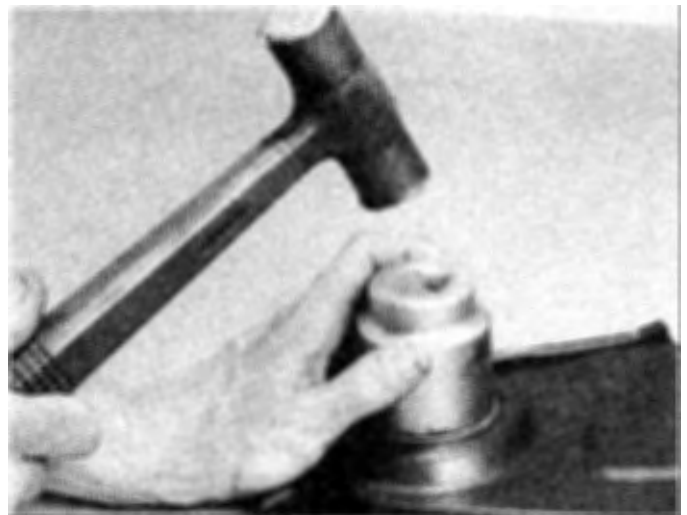
12.8a Clean the bore, then apply a small amount of oil to the outer edge of the new seal and drive it squarely into the opening with a large socket . . .
