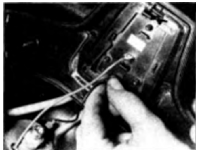
13.2 After removing the horn pad, disconnect the horn switch wires; the horn pad is retained to the steering wheel by three screws, accessible from the dashboard side of the wheel
