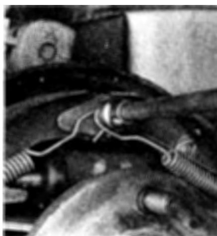
6.4e Remove the primary and secondary shoe retracting springs — the spring removal tool shown here can be purchased at most auto parts stores and greatly simplifies this step
