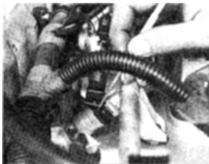
15.21b Use a scribe (shown) or a small screwdriver to pop loose the retaining clip that attaches the harness connector to each injector
