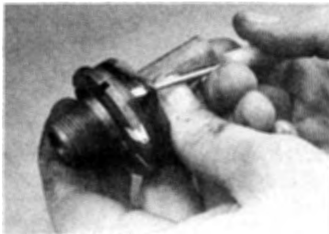
2.13a Use a small screwdriver to remove the O-ring from the groove, . . .
