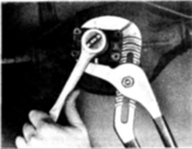
14.6b Hold the pinion shaft yoke in place and loosen the nut with a torque wrench, noting the torque necessary to loosen the nut
