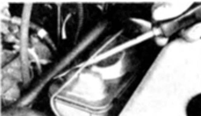
4.19b On vehicles without ABS brakes, pry the clip off the brake master cylinder cover with a screwdriver
