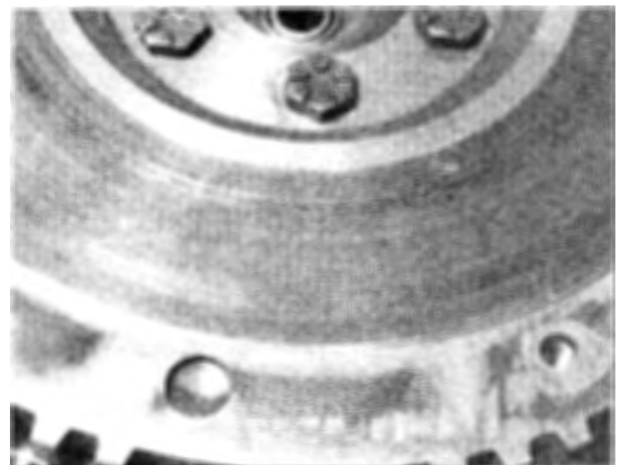
3.8 Check the surface of the flywheel for cracks, hot spots (dark colored areas) and other obvious defects; resurfacing by a machine shop will correct minor defects — the surface on this flywheel is in fairly good condition; however, resurfacing is always a good idea
