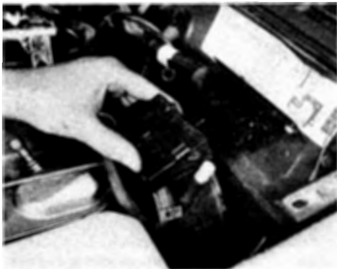
5.56 Remove the attaching screw and unplug the firewall electrical connector
