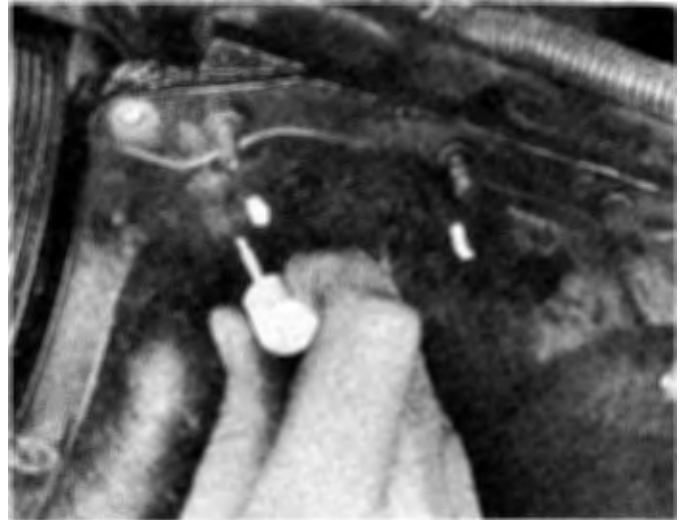
15.10 Mark the locations of the studs with paint to ensure proper reassembly
