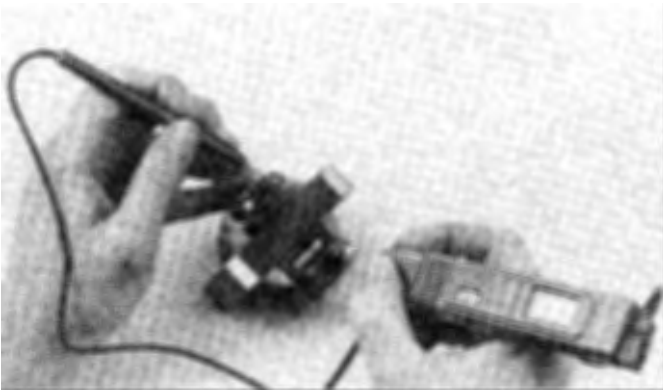
7.5 Using the high resistance scale, touch the ohmmeter negative lead to the negative primary terminal and the positive lead to the high voltage terminal — the indicated resistance should be less than infinite
