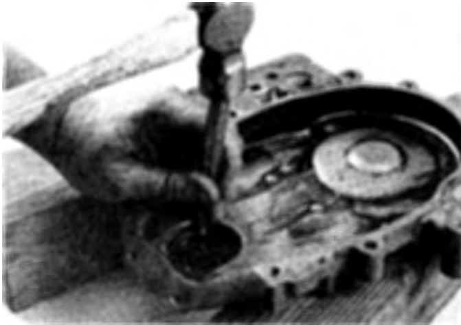
12.7 Driving the seal out of the front cover
