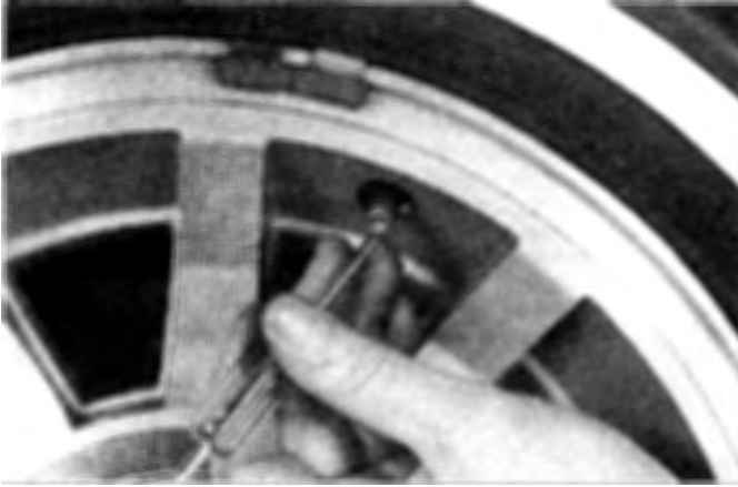
5.4a If a tire loses air on a steady basis, check the valve core first to make sure it's snug (special inexpensive wrenches are commonly available at auto parts stores)
