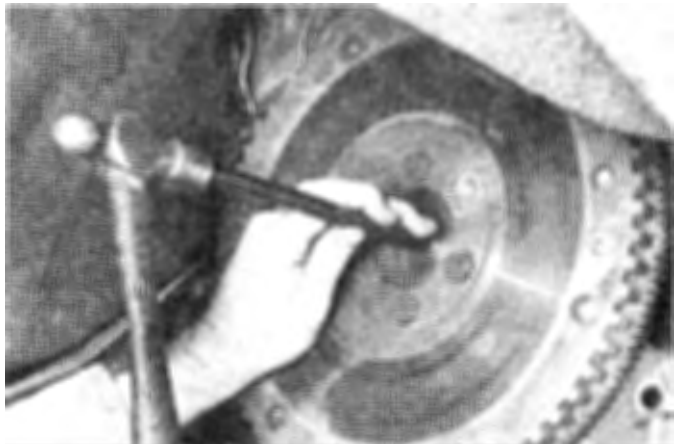
5.9 Pack the recess behind the bearing with heavy grease and force it out hydraulically with a steel rod slightly smaller than the bore in the bearing — when the hammer strikes the rod, the bearing will pop out of the crankshaft
