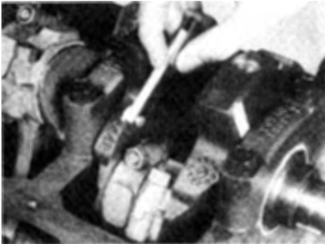
12.3 Check the connecting rod side clearance with a feeler gauge as shown
