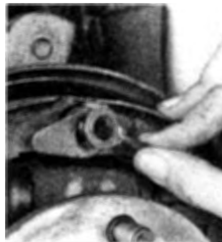
6.4f Remove the self-adjuster cable and anchor pin plate from the anchor pin
