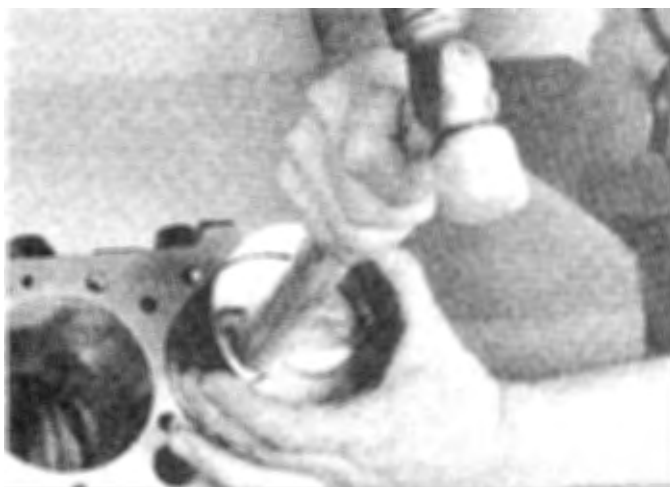
24.11 The piston can be driven (gently) into the cylinder bore with the end of a wooden hammer handle
