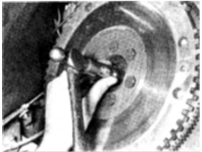
5.10b Tap the bearing in using a bushing driver or a socket
