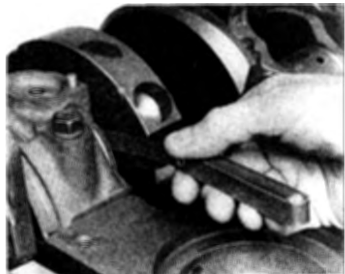
13.3 Checking crankshaft end play with a feeler gauge
