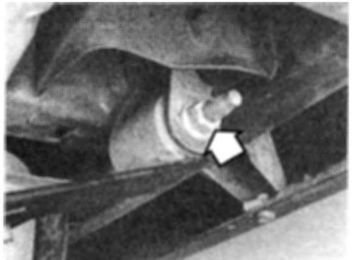
11.6 Unscrew the nut (arrow), then remove the rear spring-to-shackle bolt
