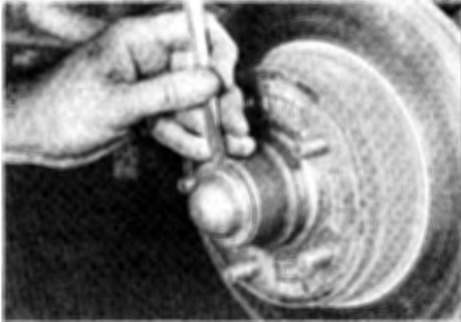
38.6 Dislodge the dust cap by working around the outer edge with a screwdriver or hammer and chisel
