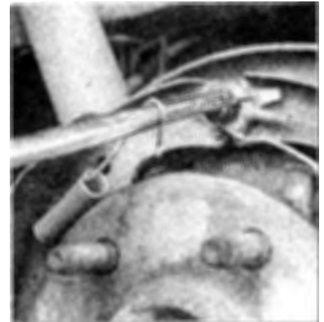
6.4u Install the primary shoe retractor spring — the tool shown here is available at most auto parts stores and makes this step much easier and safer
