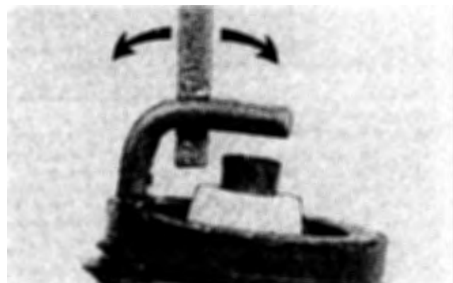
43.5b To change the gap, bend the side electrode only, as indicated by the arrows, and be very careful not to crack or chip the porcelain insulator surrounding the center electrode
