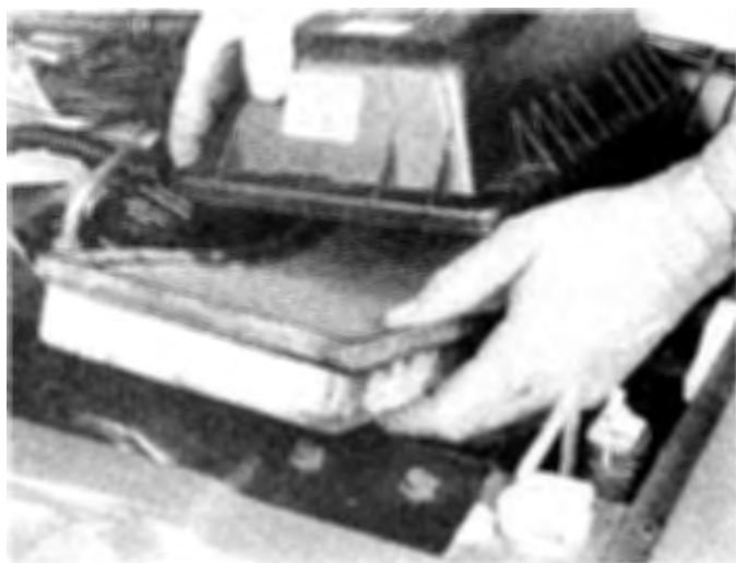
32.4 Hold the top plate up and lift the filter element out of the housing (fuel-injected model shown)
