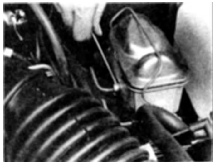
8.2 Unscrew the tube nuts from the master cylinder — use a flare-nut wrench (if one is available)
