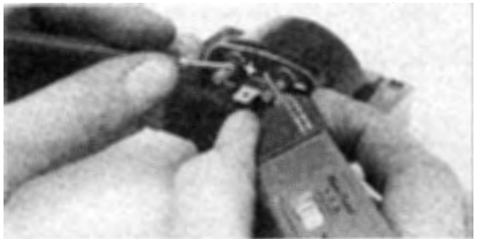
7.4 Using the low resistance scale, touch the positive lead to the positive primary coil terminal and the negative lead to the negative terminal — the indicated resistance should be zero or close to zero
