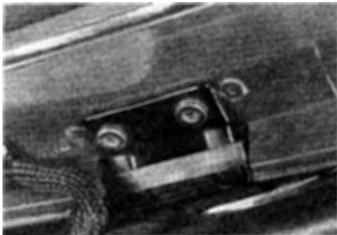
14.5 A #30 Torx head tool will be required to remove the hinge bolts
