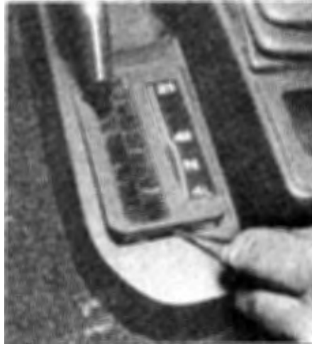
17.3b If you have a 4WD vehicle, also detach the transfer case shift plate
