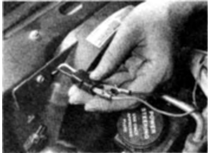
5.13 Disconnect the fan electrical connector and run jumper wires directly to the positive and negative terminals of the battery – be sure the clips don't touch each other and create a short circuit
