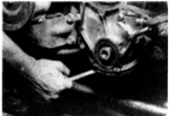
13.6B . . . and two bolts secure the timing chain cover to the front lip of the oil pan
