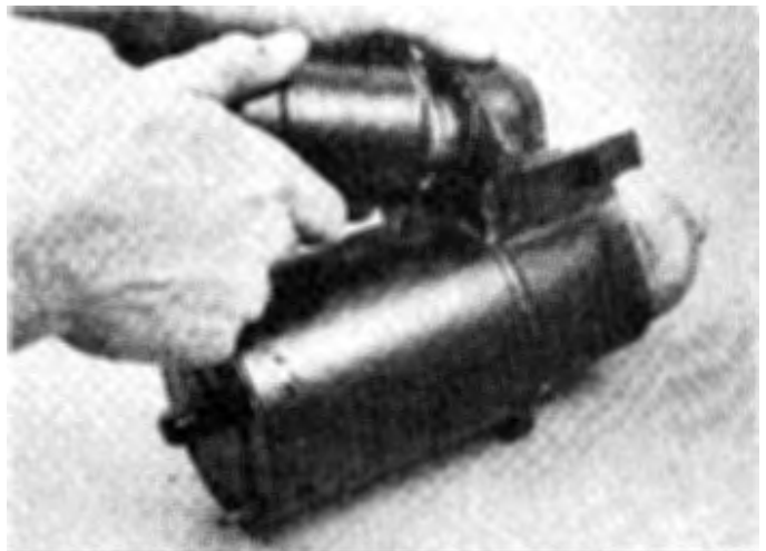
22.5 Some solenoids, like this Delco unit, must be rotated clockwise before they can be disengaged from the starter motor
