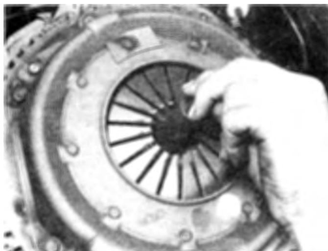
3.14 Center the clutch disc in the pressure plate with an alignment tool before the bolts are tightened
