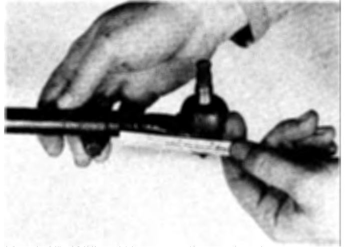
16.9 If the tie-rod ends must be replaced, measure the distance from the end of the tie rod tube to the center of the ballstud so the new tie-rod end can be set to this dimension
