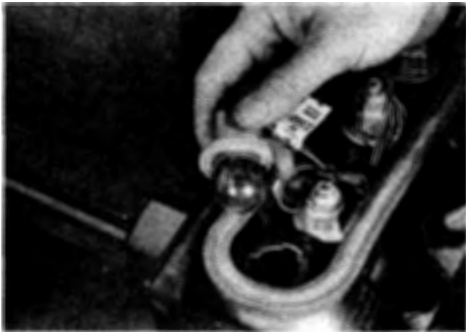
13.3 To remove a bulb housing, rotate the housing counterclockwise about 60° and pull it out
