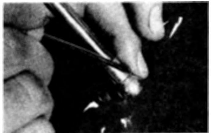
14.4 Detach the wire retainer with a small screwdriver and pry the end of the support strut off the ballstud
