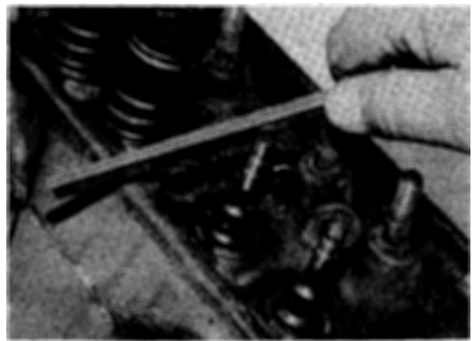
8.4 If the valve won't pull through the guide, deburr the edge of the stem end and the area around the top of the keeper groove with a file
