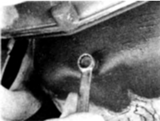
12.9 To avoid rounding off the corners of the drain plug, use the correct size box-end wrench or six-point socket to remove it
