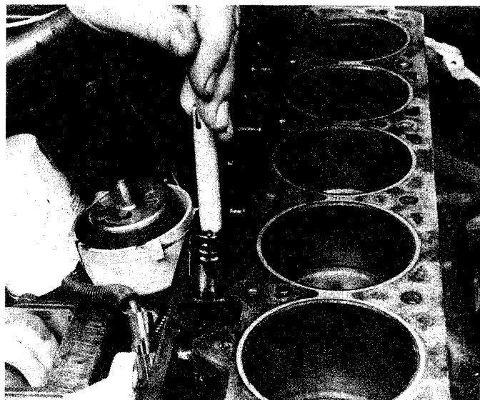
14.9 Remove the lifters with a magnetic pick-up tool (shown here) or a special lifter removal tool
