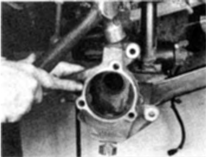
7.6 Strike the steering knuckle at the top to separate it from the balljoint studs — note that the castellated nuts are loosened, but not removed — this will prevent the knuckle from falling when it suddenly breaks loose
