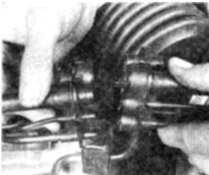
7.5 Lift the vacuum connector from its bracket and pull it apart
