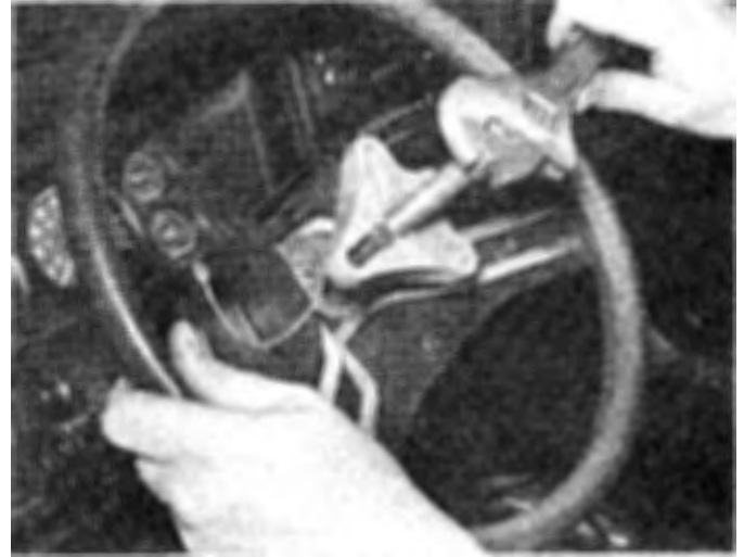
13.4 Remove the wheel from the shaft with a puller — DO NOT HAMMER ON THE SHAFT!
