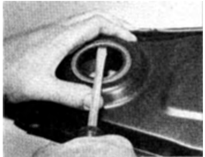
12.6 Once the timing chain cover is removed, place it on a flat surface and gently pry the old seal out with a large screwdriver
