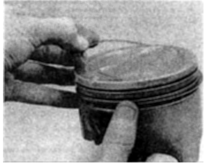
21.9b DO NOT use a piston ring installation tool when installing the oil ring side rails
