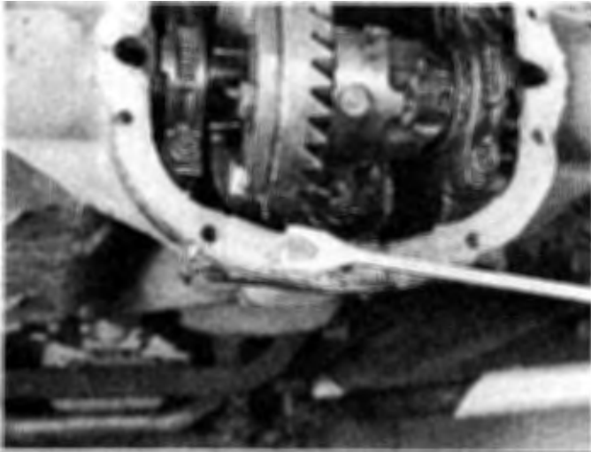
36.8 Carefully scrape the old gasket or sealant material off to ensure a clean surface for the new gasket to seal against
