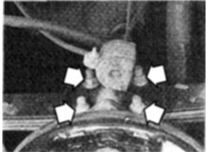
11.5 The rear axle must be supported before removing the U-bolt nuts (arrows); otherwise the axle will fall
