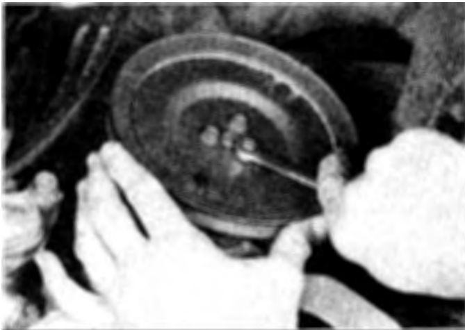
5.11 To remove the air pump pulley, loosen the three bolts, remove the drivebelt, then remove the bolts
