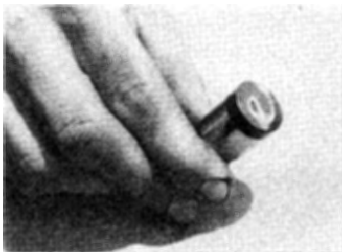
10.8a If the bottom (foot) of any lifter is worn concave (shown here), scratched or galled, replace the entire set with new lifters
