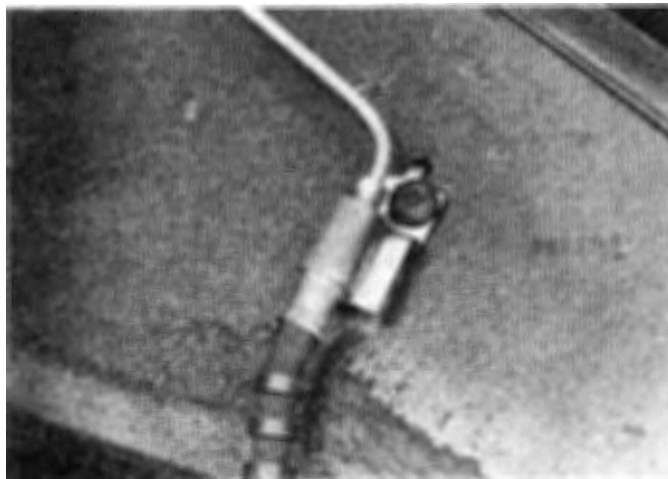
10.2 To remove the brake hose, unscrew the brake line from the hose fitting, using a flare-nut wrench; then unbolt the hose from the frame, using a Torx socket or screwdriver
