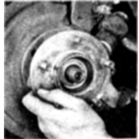
15.4b Carefully tap the hub assembly out of the steering knuckle
