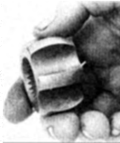
16.15a Check the inner race lands and grooves for pitting and score marks
