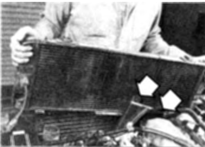
4.9 When lifting the radiator out, be careful not to damage the cooling fins with the fan and fan shroud (arrows) — inline six-cylinder model shown
