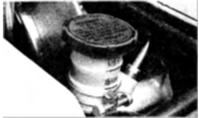
4.18 The clutch master cylinder is located next to the brake booster — maintain the fluid level between the MAX and MIN marks
