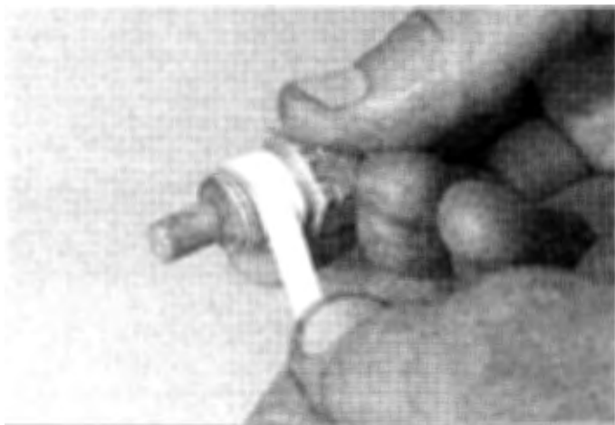
9.3 Wrap the threads of the coolant temperature sensor with Teflon tape to prevent leaks
